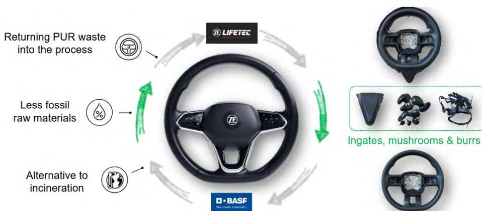
Scheme 1. Steering wheels polyurethane foam recycling running project.
